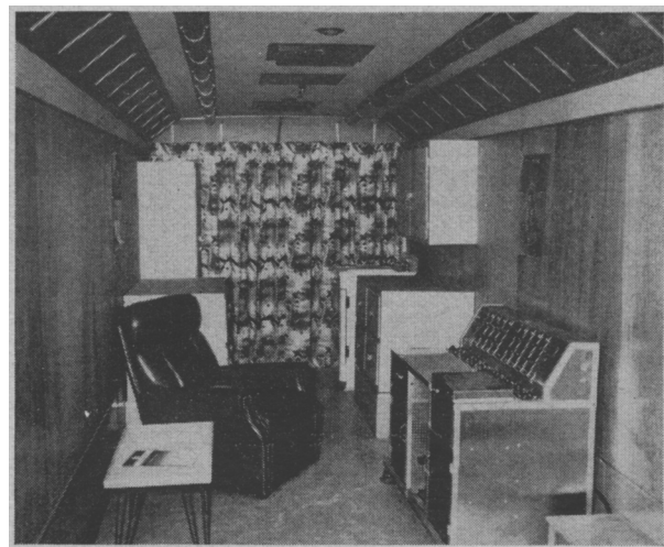
Fig. 2.—Inside of truck looking toward back from co-driver's seat. Curtain shuts off back windows. On right-hand wall are eight-channel electroencephalograph, cabinets for kitchenware above and clothes below, and combination sink, two-burner stove, and refrigerator. At left are chair used for patient during EEG, more storage cabinets, and clothes closet. By moving curtain into position behind EEG instrument, working and living quarters can be separated.
